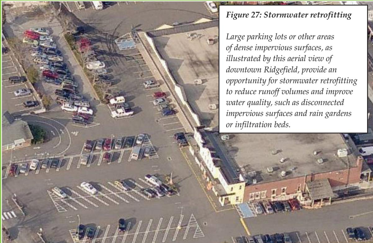
**Figure 27: Stormwater retrofitting**
