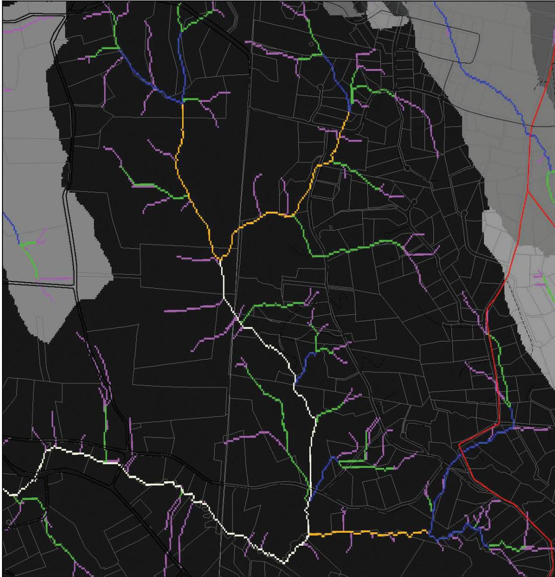
Figure 4: Stream drainage network, Mopus Brook. The shades in the background illustrate different drainage basins; only water from areas that are dark gray flows into Mopus Brook. The colors used for the brook and its tributaries represent stream order. Higher stream order indicates more tributaries. This map was created as a model, based on a digital elevation model (DEM) obtained from the National Elevation Database (prep. K. Amick).
