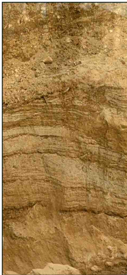
Stratified loamy sands beneath gravelly silt loam.
