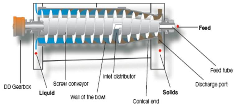
**FIGURE 7-25. THICKENING AND DEWATERING CENTRIFUGE INSTALLATION PHOTO AND PROCESS SCHEMATIC**
