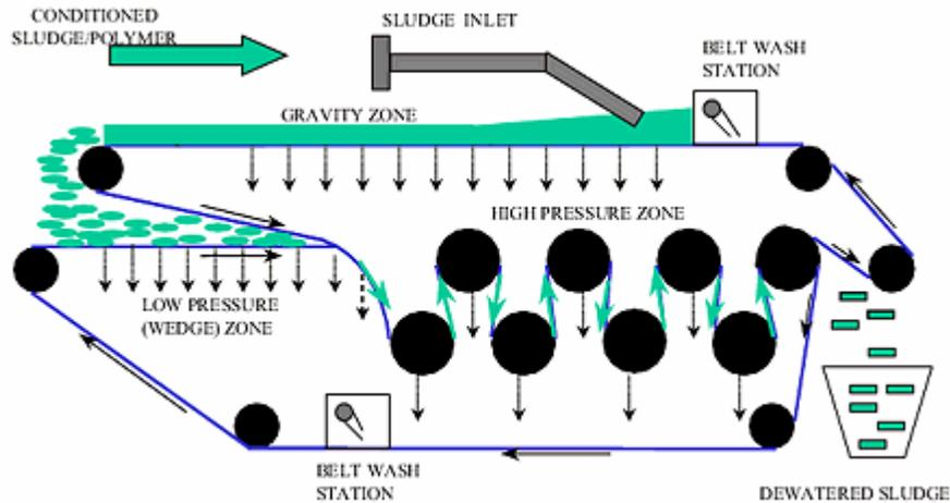
**FIGURE 7-24. GRAVITY BELT THICKENER / BELT FILTER PRESS SCHEMATIC**
