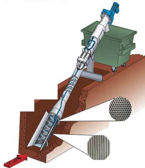
**FIGURE 6-3. ROTATING CHANNEL SCREEN**
