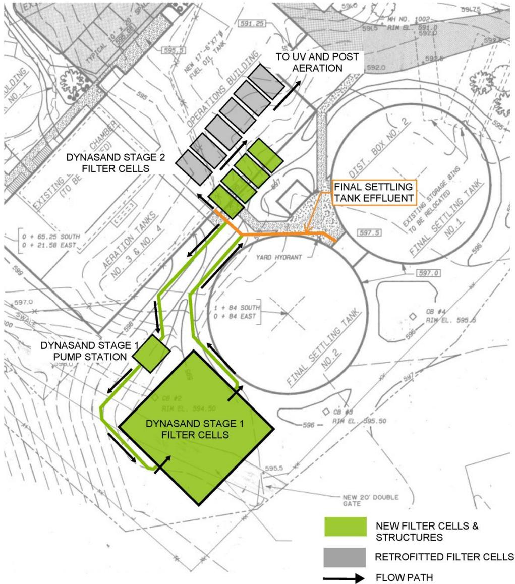
**FIGURE 7-16. DYNASAND ALTERNATIVE STAGE ONE PROCESS LAYOUT**
