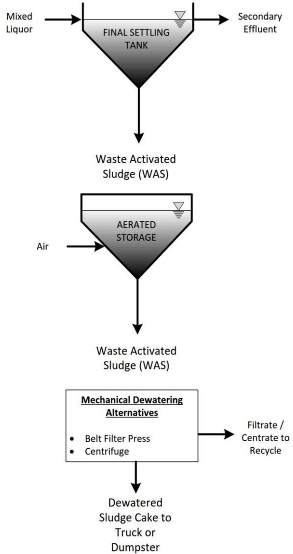
**FIGURE 7-30. BIOLOGICAL PHOSPHORUS REMOVAL SLUDGE DEWATERING SOLIDS HANDLING ALTERNATIVES**
