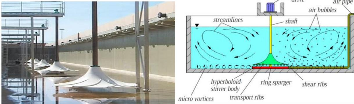
**FIGURE 7-21. INVENT MIXER/AERATOR - INSTALLATION AND PROCESS SCHEMATIC**
