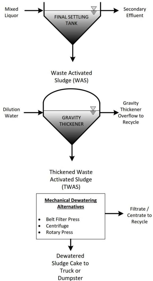
**FIGURE 7-28. CHEMICAL PHOSPHORUS REMOVAL SLUDGE DEWATERING SOLIDS HANDLING ALTERNATIVES**
