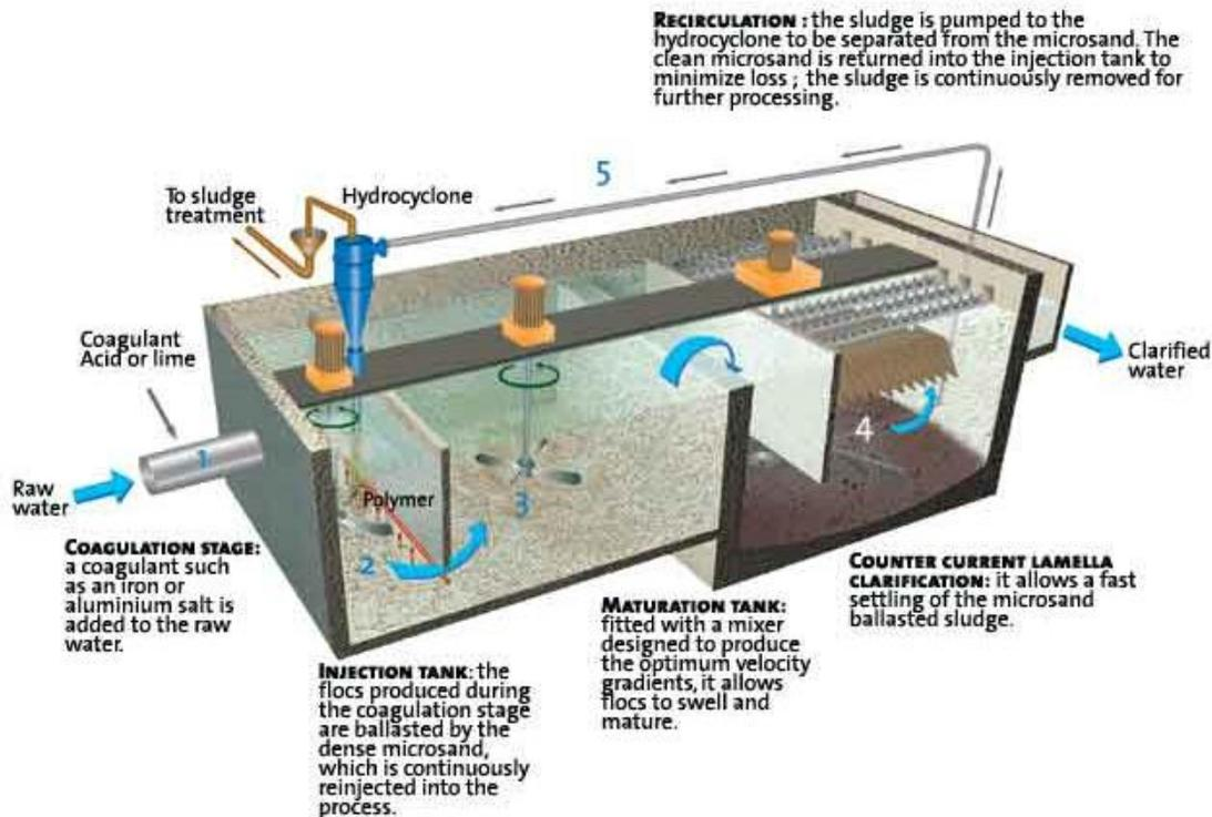
**FIGURE 7-11. ACTIFLO PROCESS FLOW SCHEMATIC**
