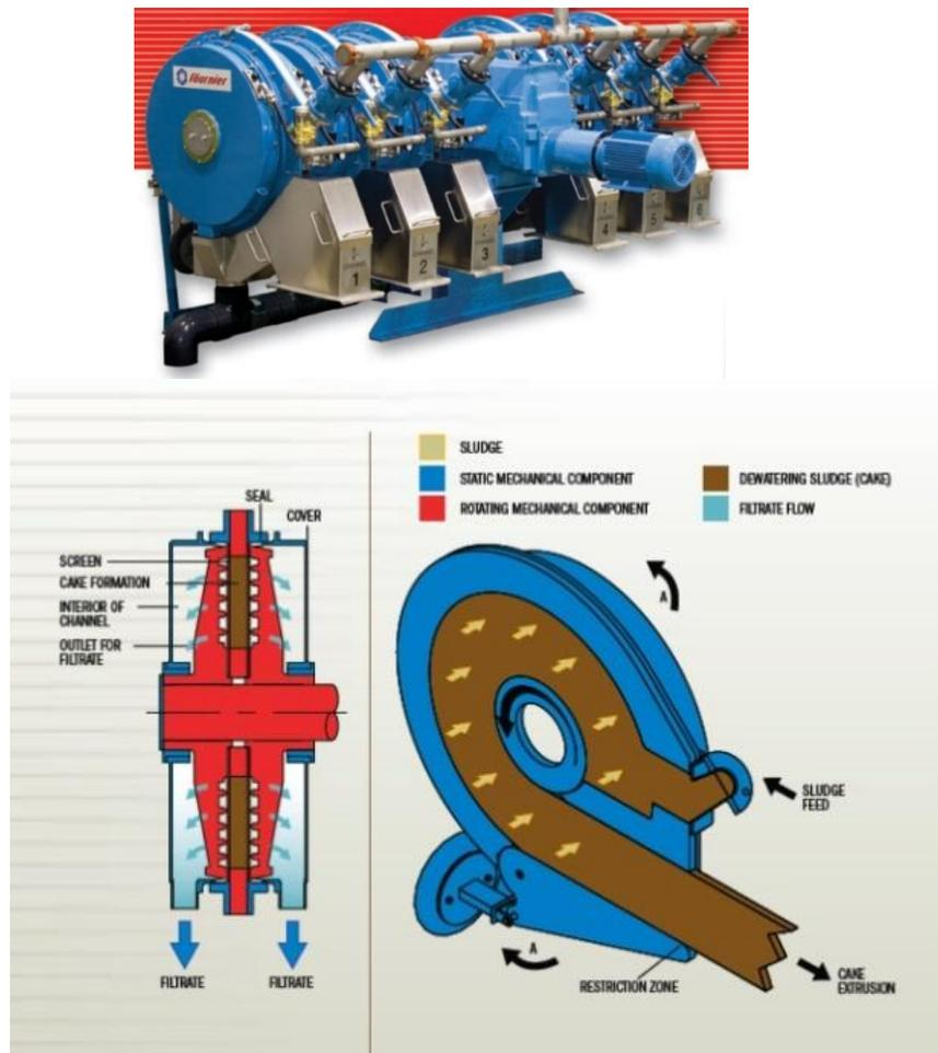
FIGURE 7-26. ROTARY PRESS INSTALLATION PHOTO AND PROCESS SCHEMATIC
