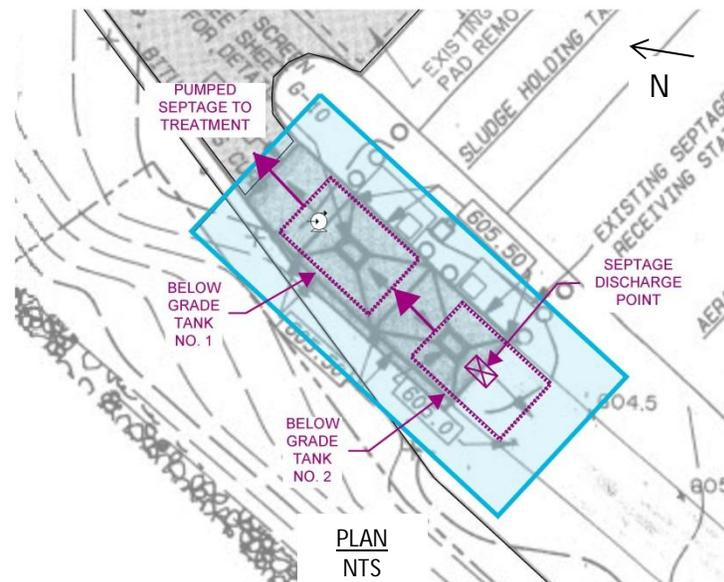
**FIGURE 7-1. SEPTAGE RECEIVING - FULL VACTOR TRUCK SIZED BUILDING**
