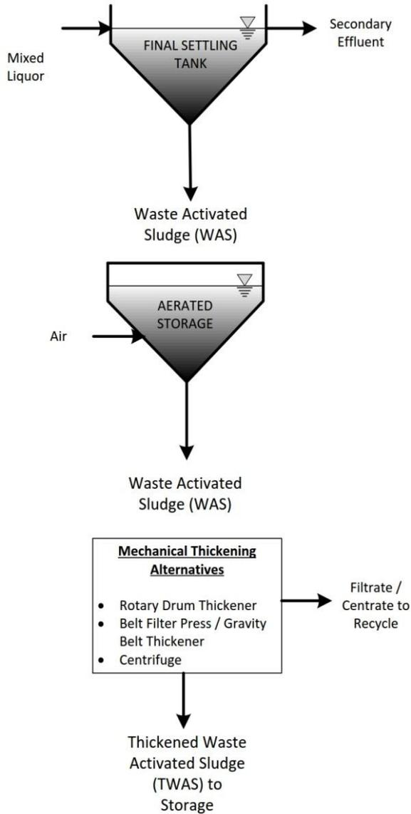
**FIGURE 7-29. BIOLOGICAL PHOSPHORUS REMOVAL SLUDGE THICKENING SOLIDS HANDLING ALTERNATIVES**
