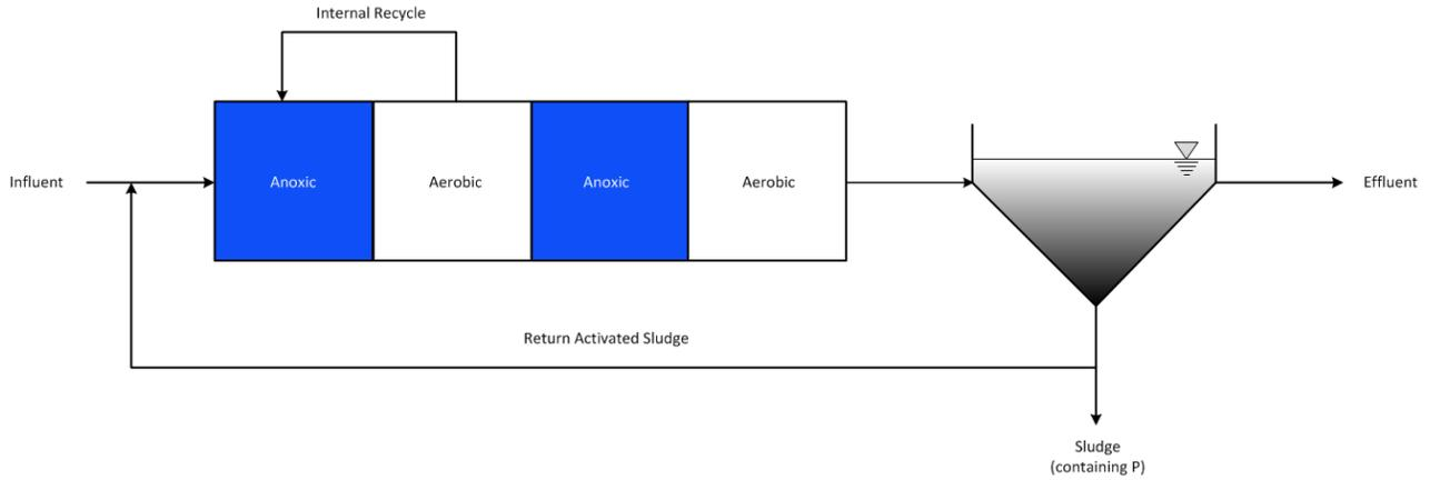
FIGURE 7-5. 4-STAGE BARDENPHO PROCESS FLOW DIAGRAM
