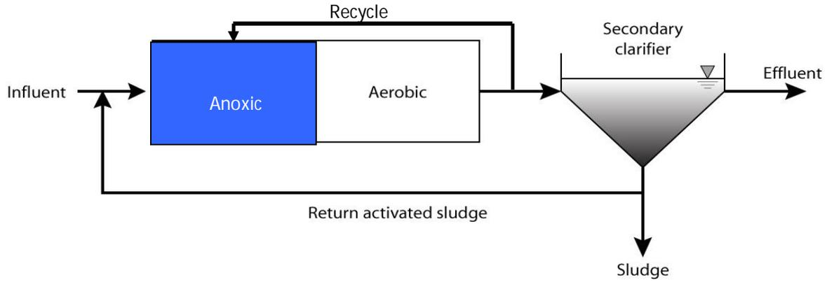
**FIGURE 7-3. MODIFIED LUDZACK-ETTINGER (MLE) PROCESS FLOW DIAGRAM**
