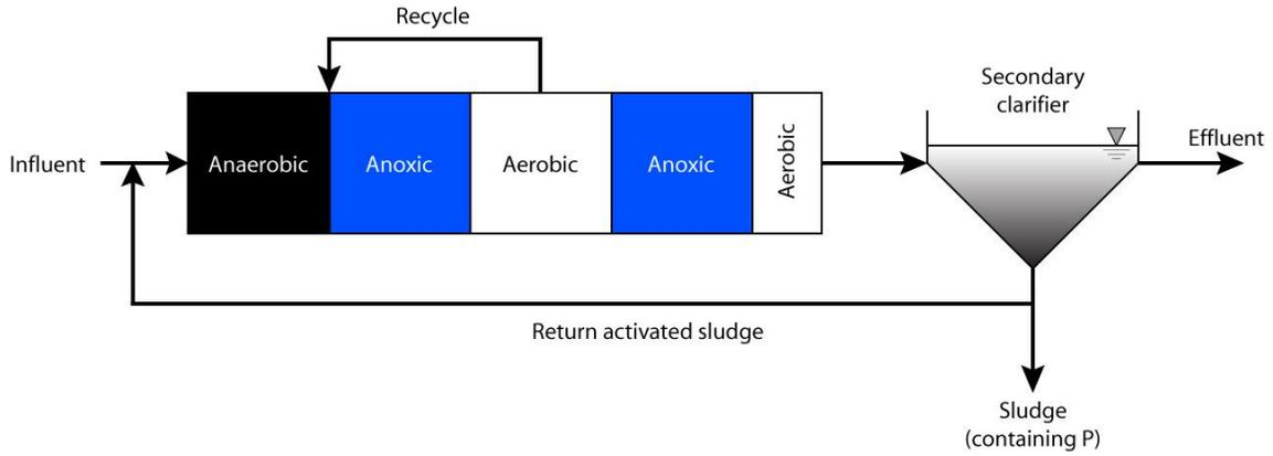
**FIGURE 7-9. 5-STAGE BARDENPHO PROCESS FLOW DIAGRAM**
