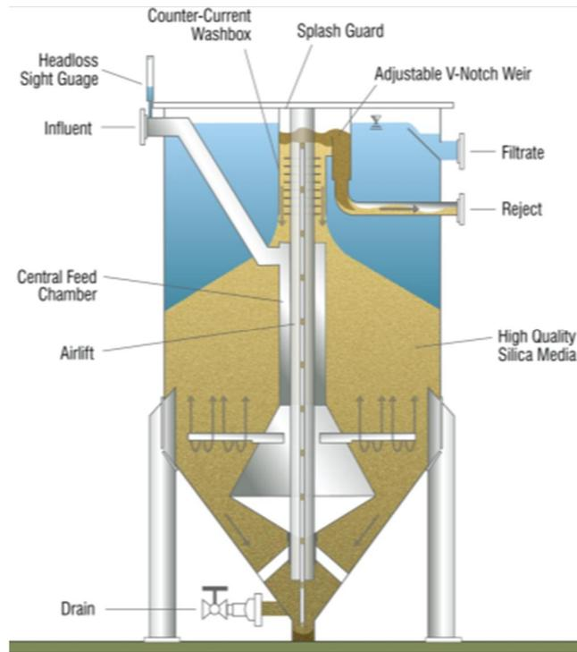
**FIGURE 7-13. BLUE PRO FILTER UNIT PROCESS FLOW SCHEMATIC**
