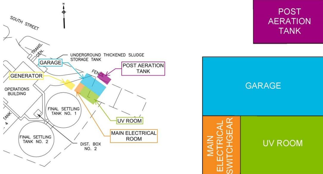
**FIGURE 9-4. RECOMMENDED UV DISINFECTION, SWITCHGEAR AND GARAGE BUILDING AND POST AERATION TANK LAYOUT**
