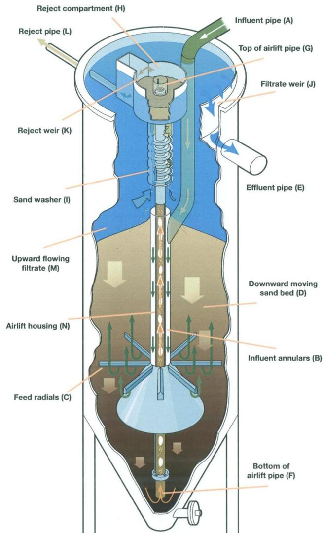
**FIGURE 7-15. DYNASAND FILTER UNIT PROCESS FLOW SCHEMATIC**
