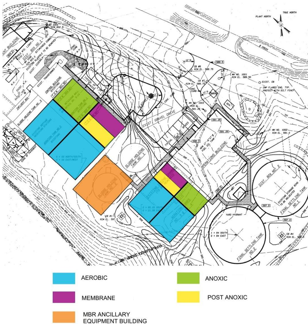
**FIGURE 7-18. MEMBRANE BIOREACTOR ALTERNATIVE PROCESS LAYOUT**
