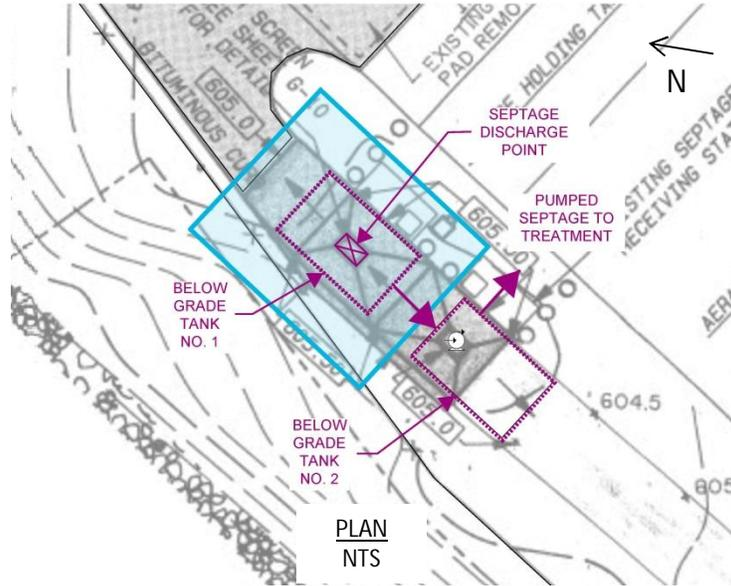
**FIGURE 7-2. SEPTAGE RECEIVING - PARTIAL VACTOR TRUCK SIZED BUILDING**
