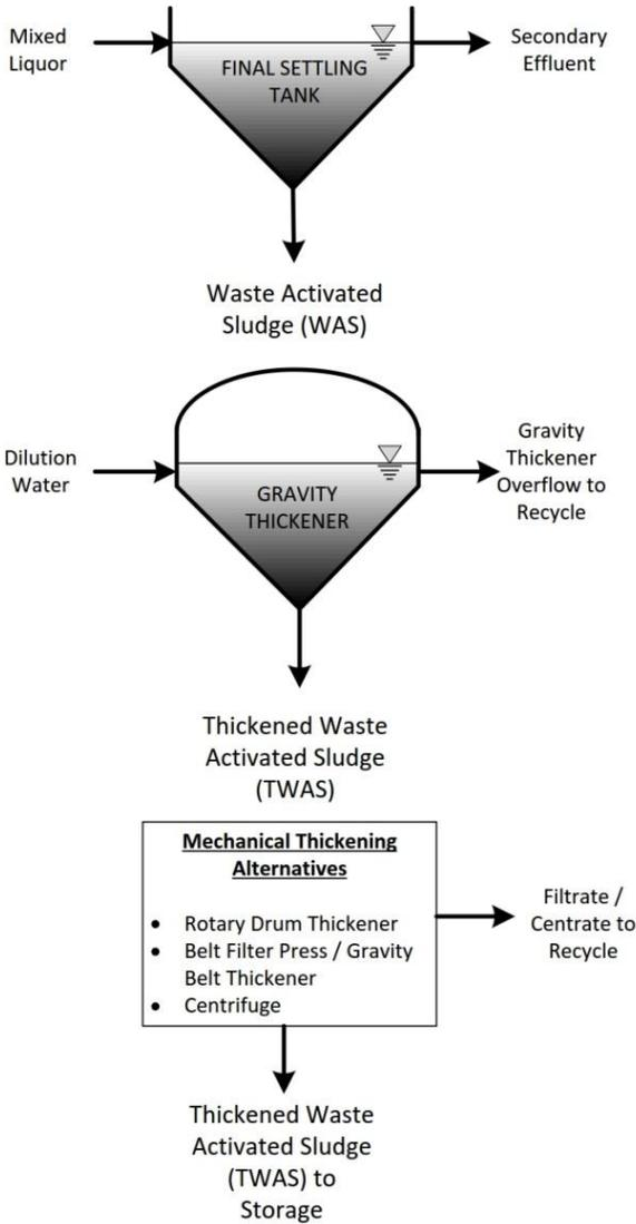
**FIGURE 7-27. CHEMICAL PHOSPHORUS REMOVAL SLUDGE THICKENING SOLIDS HANDLING ALTERNATIVES**
