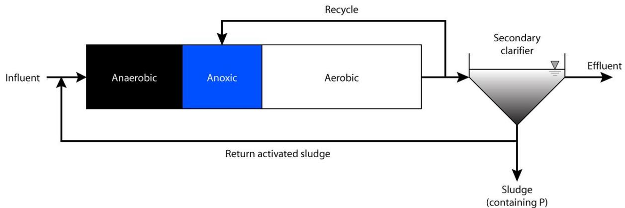
**FIGURE 7-7. A2O PROCESS FLOW DIAGRAM**
