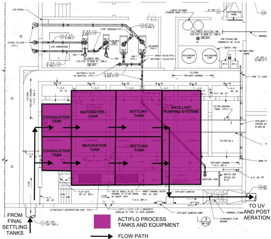
**FIGURE 7-12. ACTIFLO ALTERNATIVE PROCESS LAYOUT**
