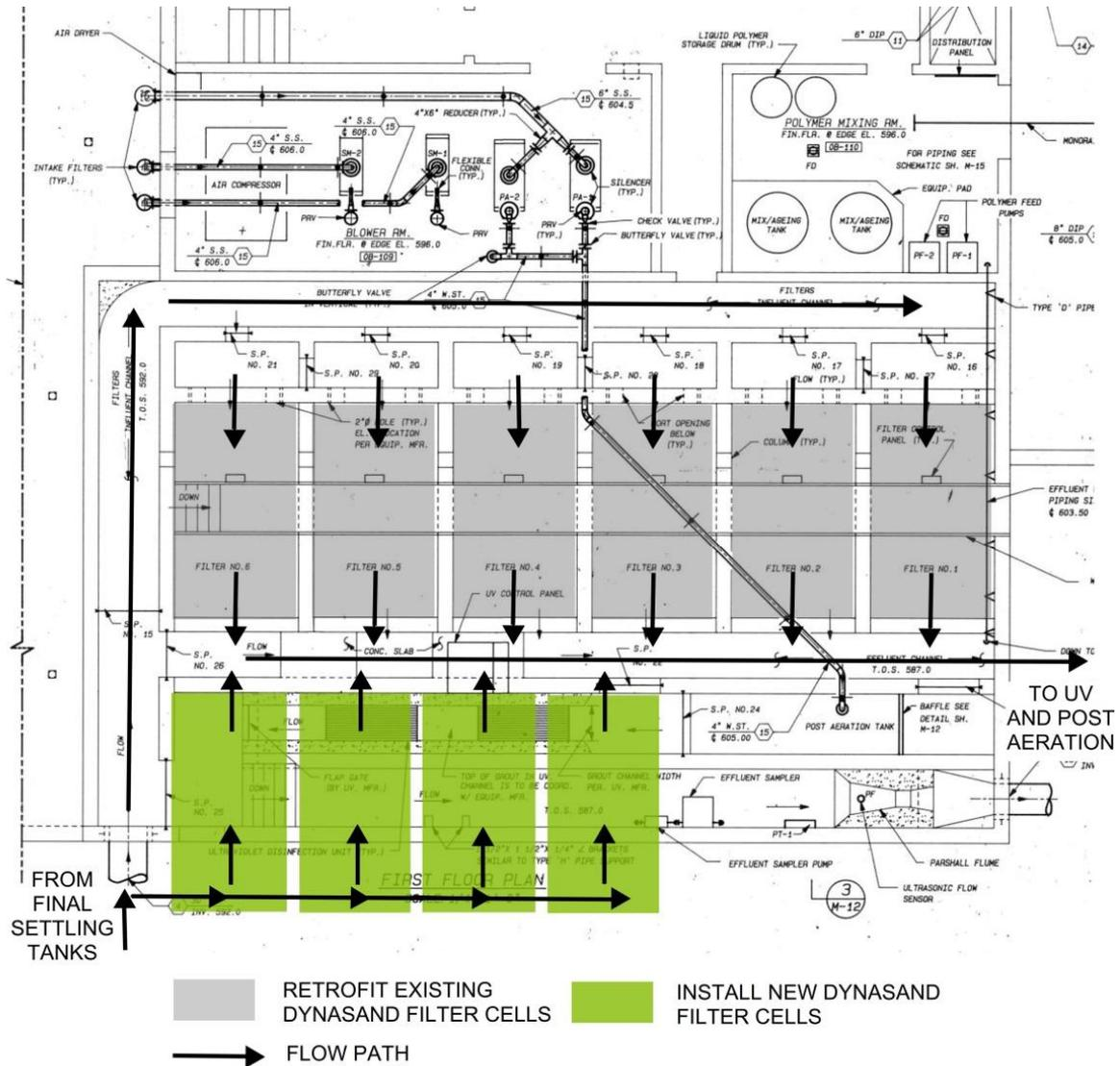
**FIGURE 7-17. DYNASAND ALTERNATIVE STAGE TWO PROCESS LAYOUT**
